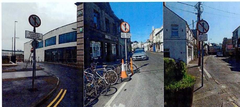
Figure: Examples from Galway of “No straight ahead” signs in operation. Left image: Station Road is closed to traffic other than buses, taxis and bicycles. Centre and right images: A section of Sea Road/William Street West is closed from two different directions – in this case the sign closes the road to all traffic at certain times. A point to note is that there do not have to be no-entry markings on the roadway.
